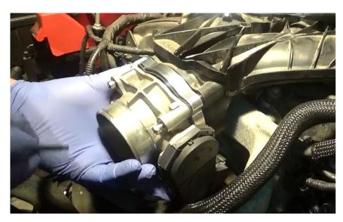
2012-15 - Remove the MAF sensor from the factory air filter housing use a torx bit. Note the included wiring extension harness to reach the new location.
