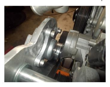
Step 8: Install Mounting Plates and Vortech Unit
