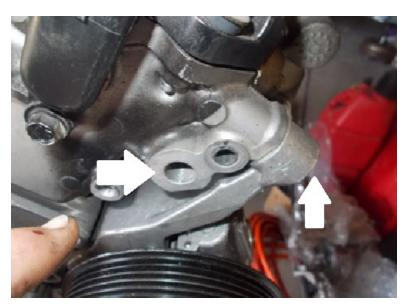
Grab the 2 M8 screws, the thick washers and the smaller diameter spacers; you're going to use these to fasten the two plates together before installing. Slide the washers on the bolts first, then pass the bolts through the backside (the side the rectangular block is attached to) of the upper holes, slide the spacers over the bolts, put a little Loctite on the threads, line up with the outer (supercharger side) plate and fasten together with the bolts finger tight.
