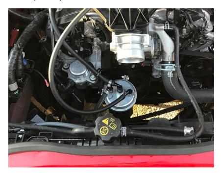
Disconnect the line that runs from the back of the passenger's side valve cover to the top of the intake manifold. There's a tab to slide sideways and the fitting will slide up and off of the PCV fitting on the valve cover. Rotate the fitting on the manifold counter clockwise and watch for the locking tabs to be released, then it can be pulled upward.
