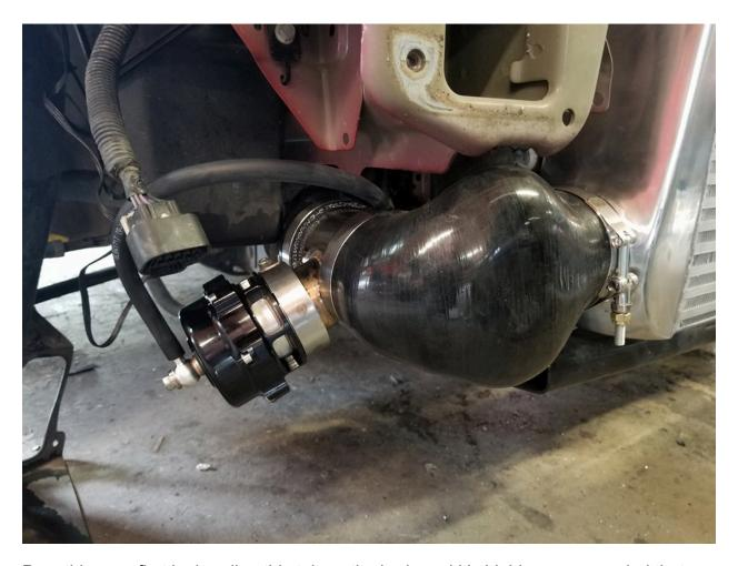
Prep this area first by bending this tab on the body and it's highly recommended that you cut the triangle tip off of the subframe to create a little more room for the tubing to pass through, but not 100% necessary. You'll see we use an electric sawzall and blade, but a good hacksaw will do perfect as well. A metal grinder......eeeehhh.....but either way, be careful to only cut what you intend to cut!
