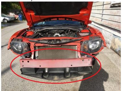
You'll also need to remove this large piece of air deflector plastic to make room for the intercooler.
