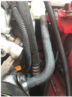
Finish with the smaller hose. It's suggested to run the hose right from the reservoir to the oil cooler up front. You can alternatively use the included 3/8" barbed hose joiner to secure to the hose end that you took out of the factory reservoir. If the former, remove the 10mm bolt securing the old hose next to the radiator, and remove. Trim the hose to desired length and route/secure as desired away from moving parts.
