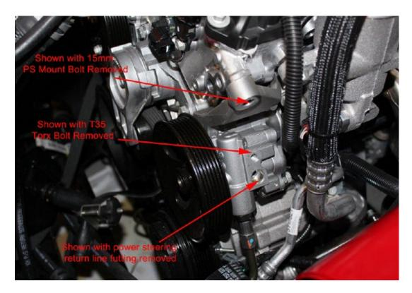
We'll now begin to install the new power steering reservoir system. Start with the new pump fitting, it's a one piece fitting with an Oring installed, and a C-clip retainer plate. Install the fitting in the pump, slide the retainer plate inplace and secure with the new bolt included (or you can use the old Torx bolt).
