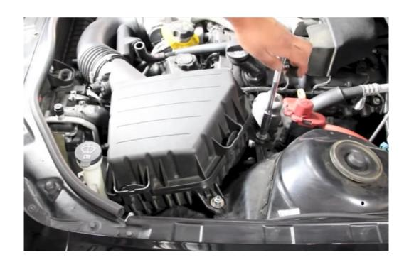
Step 4: Install new Power Steering Reservoir System
