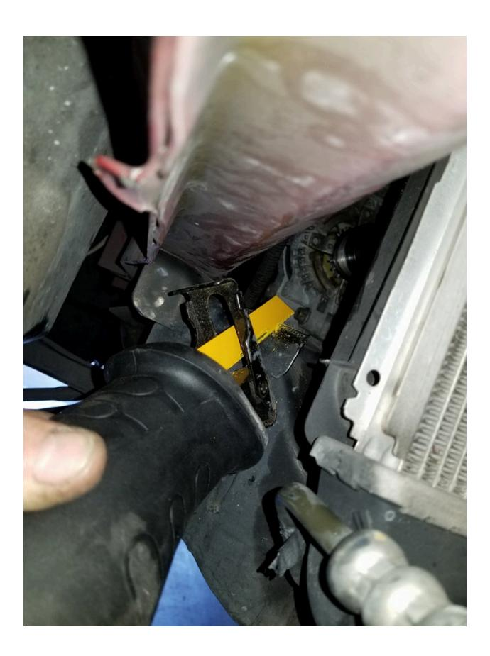
Start by sliding the long preformed silicone tube down from inside the engine bay until it pokes through to the fender well, you can use some WD40 spray on the outside of the silicone tube to help glide it past the subframe to where it needs to be. Next, preassemble the BOV valve tee into the Cobra head 90\* elbow, it goes into the short end of the head, with a clamp.
