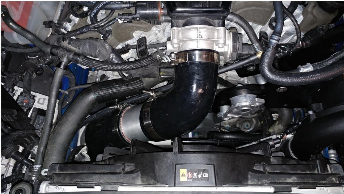
Now is a good time if you've not done so yet to take the 1/4" hose from the BOV throttle body spacer kit and run it from the spacer to the BOV vacuum fitting on its top.
