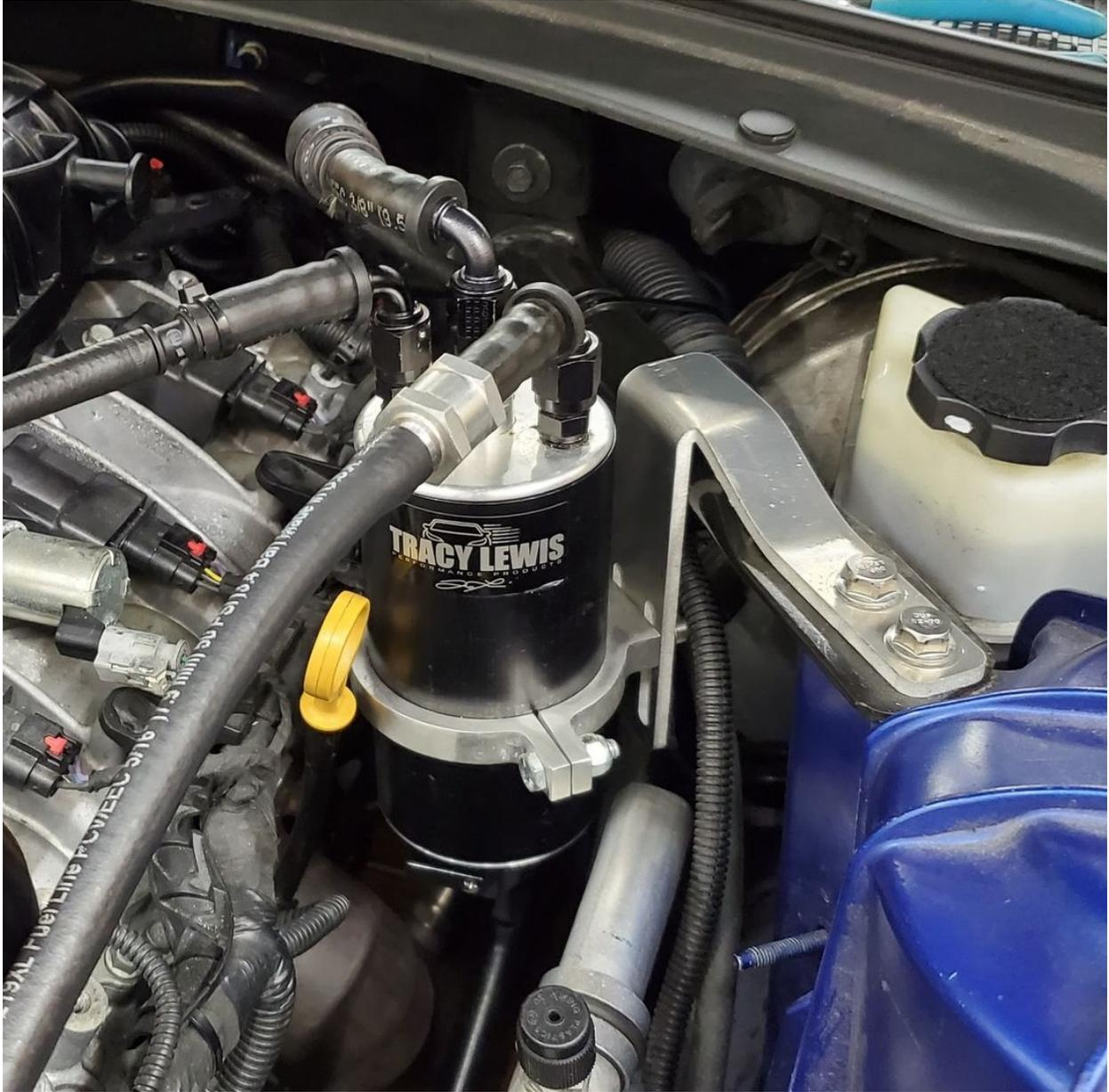
Line #1 connects to the large hard plastic running the length of the intake manifold on the driver's side. The line has a short length of the large 5/8" size and reduces to 3/8"; connect the larger end to the plastic factory line and then run in a cosmetically pleasing fashion over to the center port on the catch can, trim its length as you desire with a knife or scissors and slide it over the center port barb.
