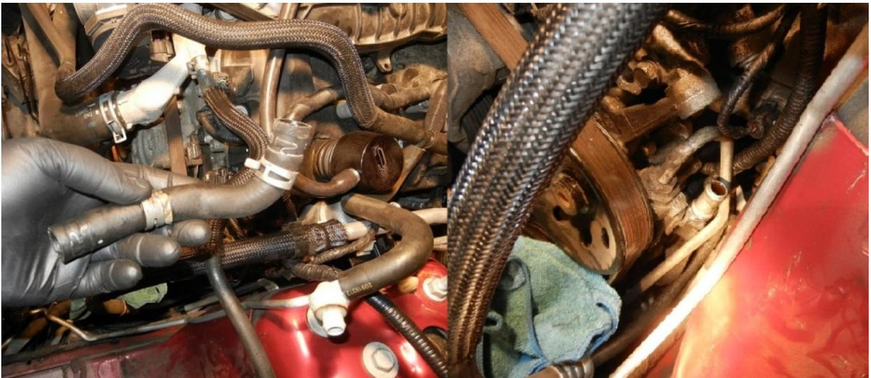
The new reservoir mounts back beside the brake fluid reservoir. The black bracket and its aluminum sub bracket goes over the stud and is secured by the same nut. The reservoir then slides down onto the black bracket. You'll need to use a little persuasion on the A/C line to give the reservoir some clearance.
