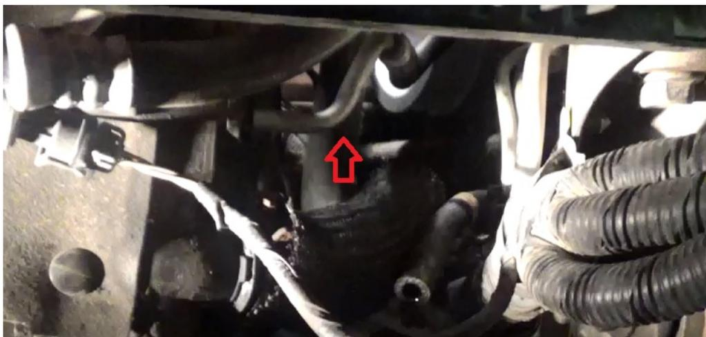
If you have a 2010-2013 model with the engine computer in the fenderwell, remove the computer from its bracket by unclipping it at the top, and follow its wiring harness to unclip and move it out of the way. You'll also want to remove the two nuts holding the bracket in place, remove the bracket, then reinstall the nuts. Set the computer aside for now, it'll be reinstalled later with its bracket in a different location.
