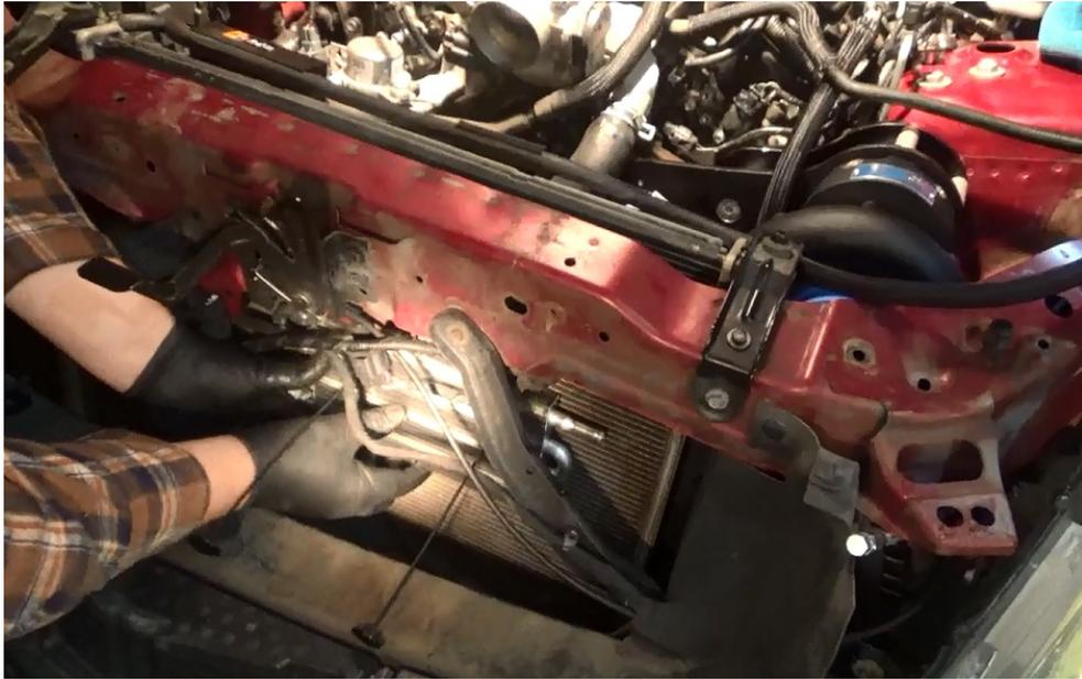
You can now secure the new cooler lines or leave it to later. You'll be running the smaller hose from the reservoir through the headlight area to the top of the cooler, leaving enough slack to run around the impending supercharger bracket install. Cut the hose to length and secure with hose clamp provided. Next run the remaining hose from the lower cooler port to the hose in the engine bay you disconnected, using the included brass barb and hose clamps to secure.
