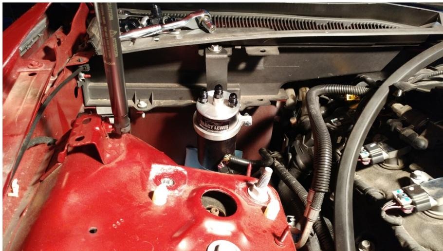
Disconnect the line that runs from the back of the passenger's side valve cover to the top of the intake manifold. There's a tab to slide sideways and the fitting will slide up
