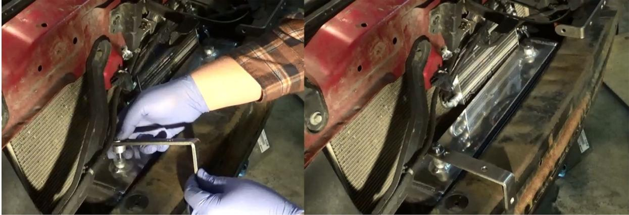
Prep to install the driver's side tubing. The small transmission cooler and A/C lines along the driver's side of the radiator will almost all need to be disconnected from their securing tabs in order to wiggle around and provide clearance.
