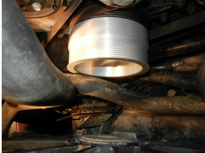
You should now find that the lower coolant hose is either touching the crank pulley or is very close. This is corrected by loosening the upper clamp on the coolant hose, and grab and twist the hose on its metal neck until you see clearance from the crank pulley of at least a finger width. Reinstall the clamp to secure. Done.
