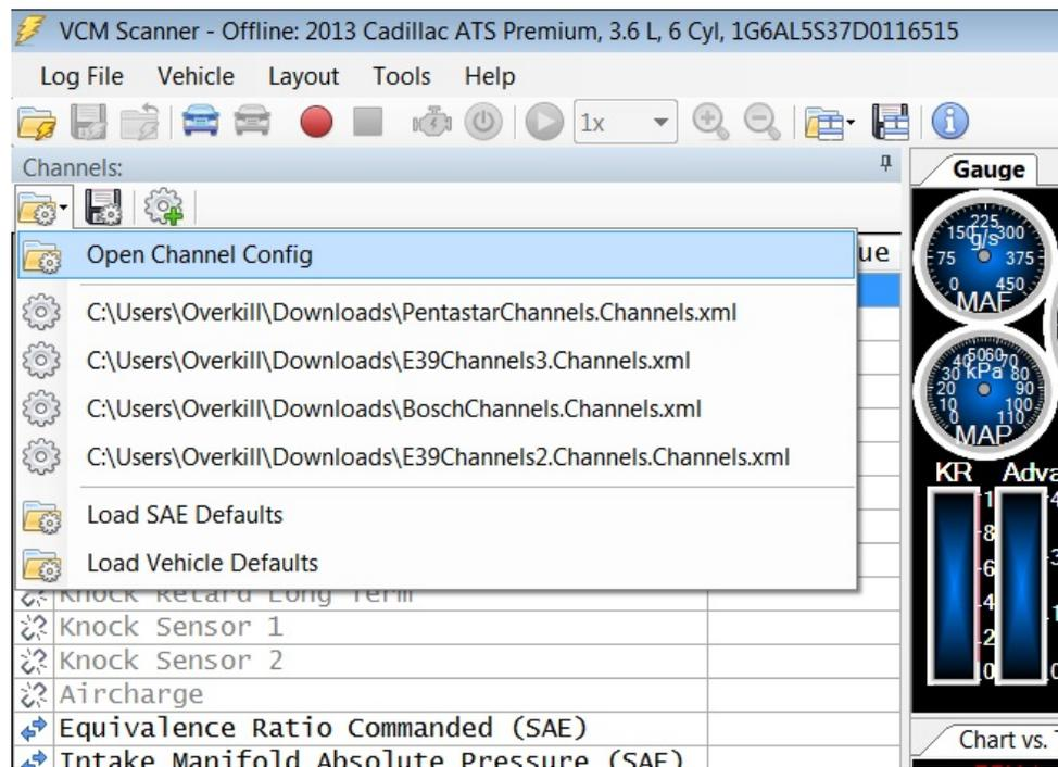
Now go to Vehicle > Connect and Vehicle > Start Scanning, confirm that you see the parameters on that table in the right hand column changing as it gets information from the computer.
