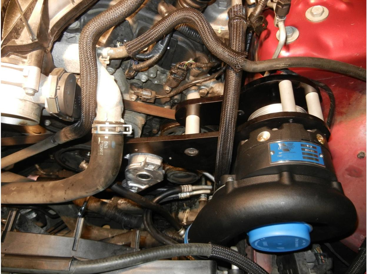
If you need to clock the Procharger, you're able to move it by loosening the 6 small allen head retaining bolts and rotating the snail like outer housing. The outlet should be pointed straight down.
