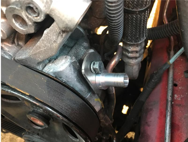
Next, mount the bracket for mounting the new fluid reservoir. Go back to the brake master cylinder; from the engine side, remove the nut securing the master cylinder to the brake booster. Slide the new bracket in place over the stud, and note the two forks fitting around the casting to prevent the bracket from rotating. Reinstall the nut.
