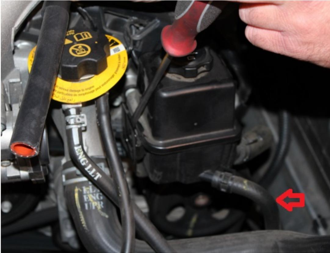
Begin by draining the reservoir of fluid. Remove the smaller hose from the reservoir and use a tub, cup or bottle to catch the fluid (tip: keep the cap on to slow the initial drain of fluid from the reservoir, then remove the cap to accelerate draining). Lower the hose to catch as much fluid from inside as possible, then push aside. Remove the larger hose from the reservoir and do the same.
