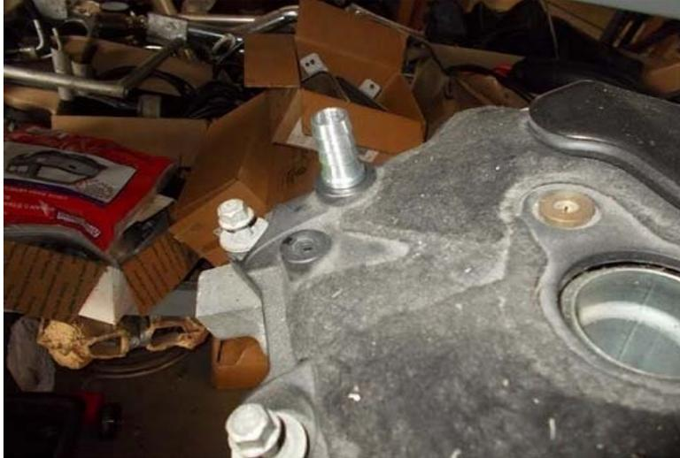
Line #2 – Install the longer 3/8" hose into the intake manifold, it will have the same factory fitting as the factory tube you previously removed. Remember to rotate the fitting to ensure the fitting is fully inserted and secure. Run to either of the outer ports on the catch can.
