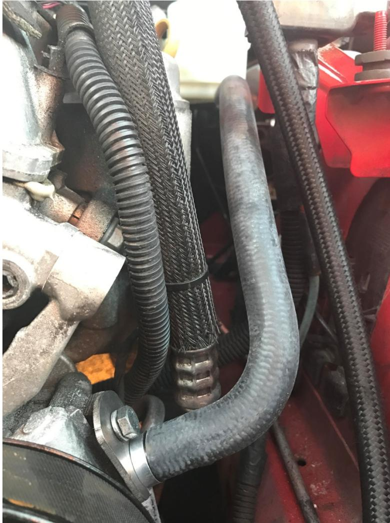
Finish with the smaller hose. You have two options, use the included barb fitting to secure to the existing hose end that you took out of the factory reservoir, or run the new hose all the way to the front of the car and secure to the cooler with no joints. If the latter, remove the 10mm bolt securing the old hose next to the radiator, and remove. Trim the hose to desired length and route/secure as desired away from moving parts.
