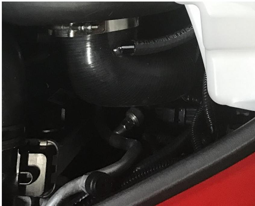
Attach the Amsoil air filter to the large aluminum elbow. Install the two regular hose clamps over the Cobra head shaped silicone intake elbow and install onto the inlet of the supercharger, do not tighten yet. Ensuring to check clearance from the A/C line, slide the aluminum elbow up from the fenderwell and into the Cobra head elbow. Once you're happy with the alignment, tighten down the clamps.
