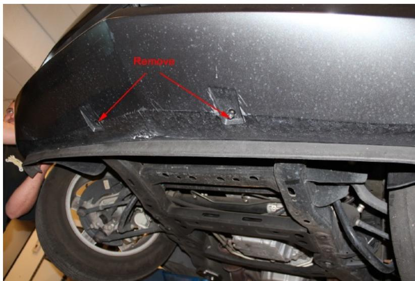
Remove the screws that line the inner fenderwell skirt and peel back (Tip: Turn the wheels to aid access to these screws), then remove the bolt marked #4 In Photo
