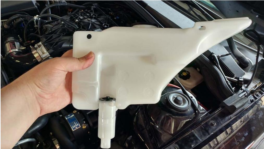
Now put the washer bottle in place, secure to the brackets using the nuts, washers and bolts provided, then tighten up the brackets once you're happy with the positioning. Plug in the fluid hose and electrical connector.
