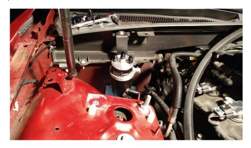
There are 4 lines to be run in total, plus a PCV valve fitting to replace. Follow along in the sequence step by step, reread as many times as you need to, and you'll be able to install the catch can successfully.
