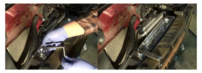
Prep to install the driver's side tubing. The small transmission cooler and A/C lines along the driver's side of the radiator will almost all need to be disconnected from their securing tabs in order to wiggle around and provide clearance.
