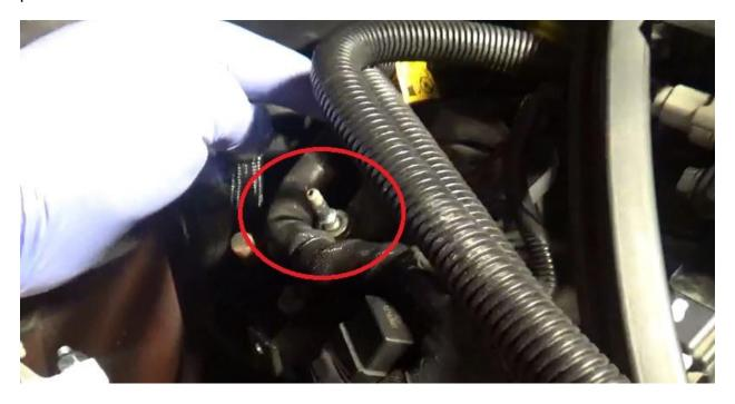
Line #1, take the short ½" hose and run it from the new valve cover fitting to the larger center port on the catch can.
