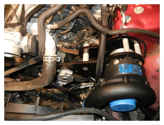
If you need to clock the Vortech, you're able to move it be loosening the 6 small allen head retaining bolts and rotating the snail like outer housing. The outlet should be pointed straight down.
