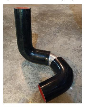
Slide the long leg tubing up by the radiator into the engine bay and with a bronze nut clamp over the end slide up and attach to the Vortech outlet. Some WD40 is helpful to slide the silicone parts onto metal, and the WD40 will dry up shortly after. Ensure you get the clamp high enough that it clamps over the top of the silicone where the reducing insert goes; if you clamp it too low it won't clamp over the insert and may come loose.
