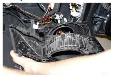
7. Unplug the TCM by sliding the lock towards the back of the car and pull the plug straight out.
