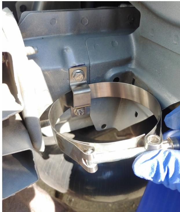
Now slide the pump into the clamp to the position you had test fit and secure the clamp, the pump should now be safely secured.
