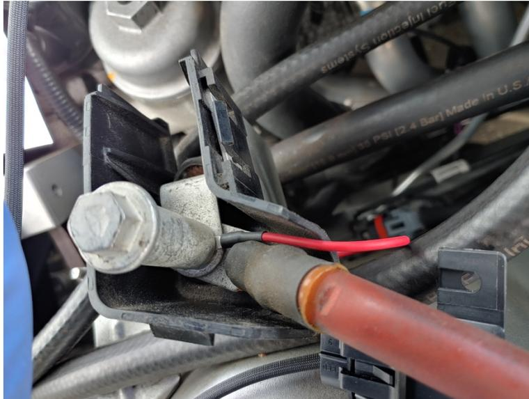
Back in the fenderwell, plug in the pump. The longest section of wire, run it over the engine in a neat fashion to the pressure switch; unplug the coil terminal closest to the pressure switch you mounted, plug the inline connection but leave the connector for the pressure switch unplugged for the moment, you'll plug it in to complete the install after we prime the system.
