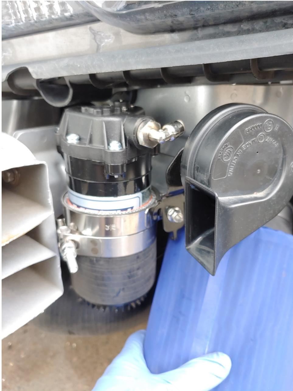
Remove horn and its bracket, unplug and set aside for now. The U shaped bracket will mount to the frame securing the clamp inside it, while the pump slips through the clamp itself; there's adjustability there to slide the pump up and down to get the pump in the position you want it.
