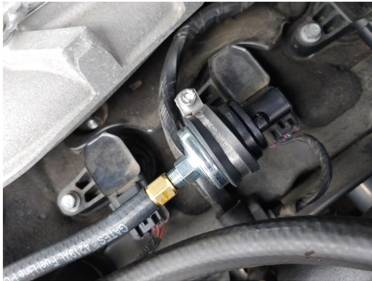
Tie the pressure switch into the BOV vacuum line. Use the included T fitting and hosing to tee into the BOV line and run to the barb fitting on the pressure switch.
