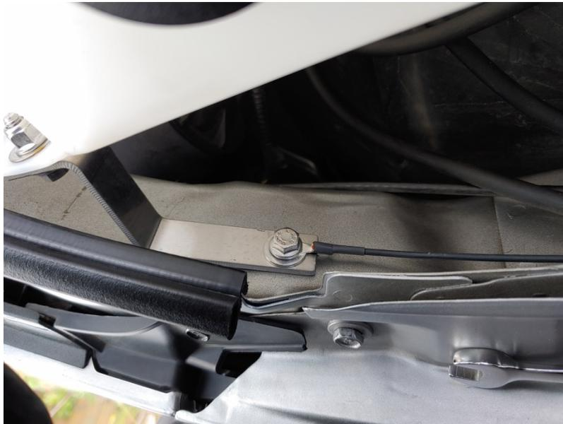
Connect the power wire beneath the nut on the power cable terminal on the driver's side strut tower.
